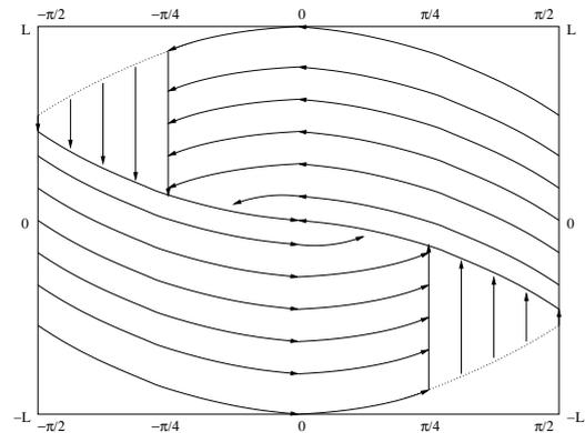
Fig. 3. The suboptimal synthesis for the Dubins' Car
