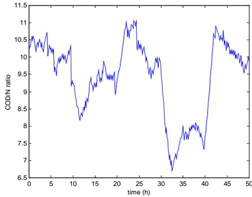
Fig. 4. Response of the process to set-point changes: COD/N ratio in the inlet of bioreactor.
