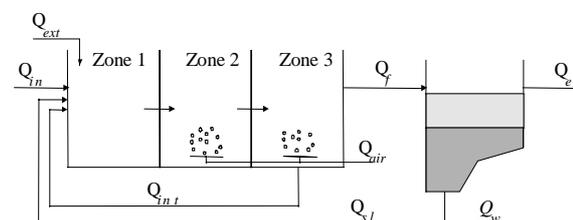
Fig. 1. Layout of the ASWWTP-USP benchmark
