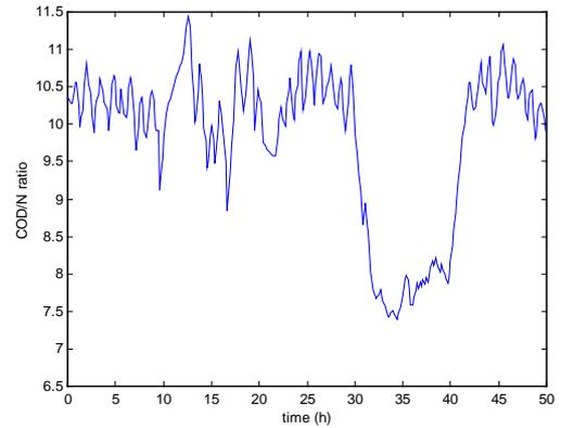
Fig. 7. Response of the process to set-point changes: COD/N ratio in the inlet of bioreactor.
