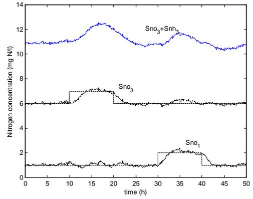
Fig. 5. Response of the process to set-point changes: controlled variables.
