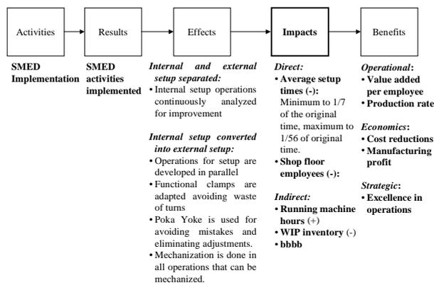
Fig. 4. Logic model of manufacturing practice: SMED (Single Minute Exchange of Dies)
