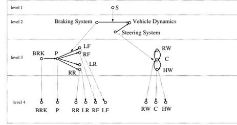
Fig. 7. A hierarchical fault propagation model for a braking and steering systems.
