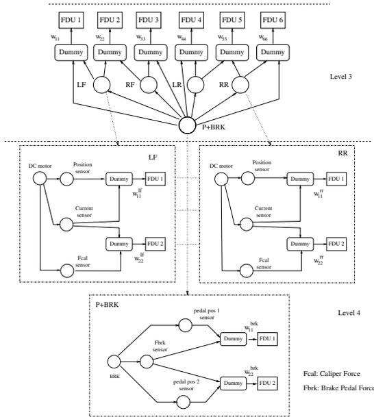
Fig. 9. Level-structuring digraph for brake system.
