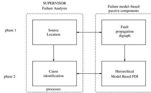
Fig. 1. A framework for model-based failure analysis.
