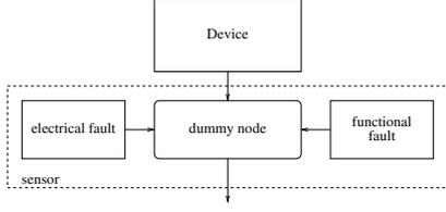
Fig. 3. Fault propagation digraph for a sensor.
