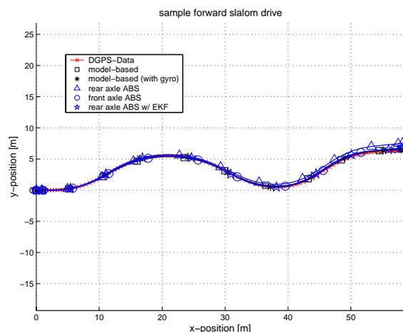
Fig. 5. Trajectory of the vehicle for a simple forward slalom drive
