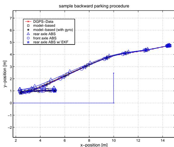
Fig. 7. Trajectory of the vehicle during a backward parking process
