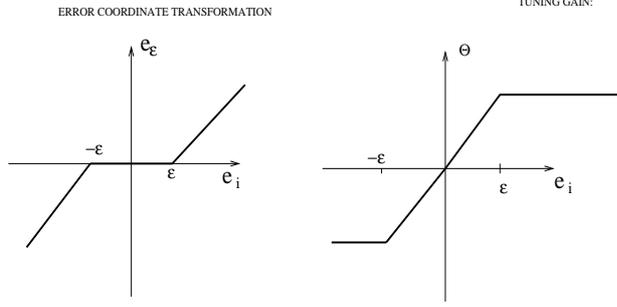
Fig. 2. Error coordinate transformation and the tuning gain used for adaptive algorithm
