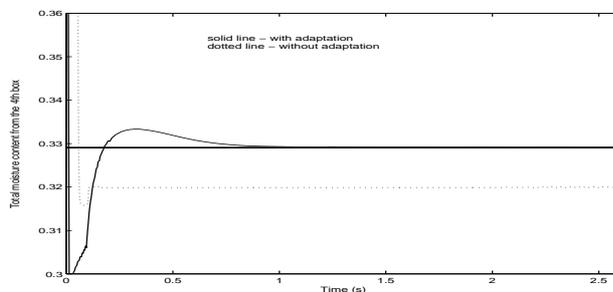
Fig. 4. Nominal and achieved total moisture content when 25% error in the process model - parameter  $K$  is introduced, with and without adaptation
