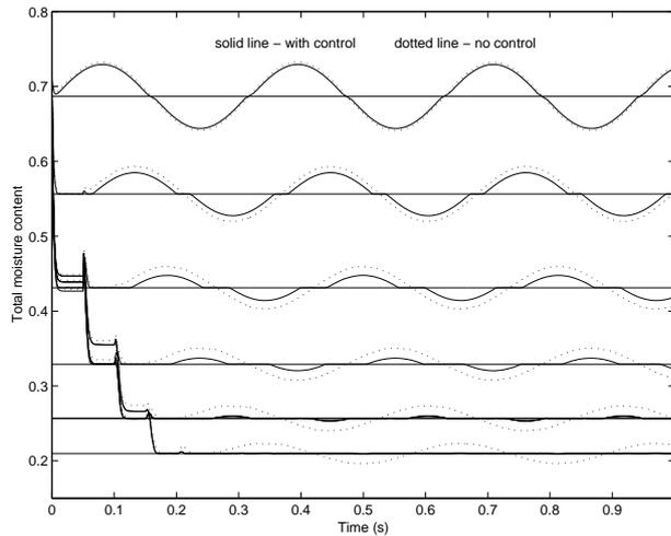
Fig. 3. Desired and actual total moisture content ( $w_i$ ,  $i = 1, \dots, 6$ ) with sinusoidal moisture content disturbance from headbox, with and without the nominal preemptive control.  $K_i$  are assumed well known.
