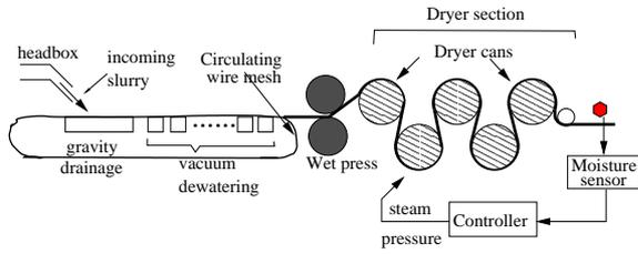
Fig. 1. Schematic of a water removal processes in a paper machine and the current process control strategy
