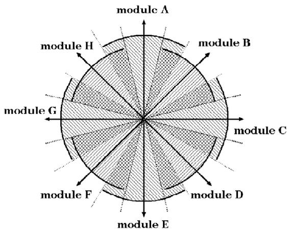
Fig. 7. The communication area of the infrared transceivers.
