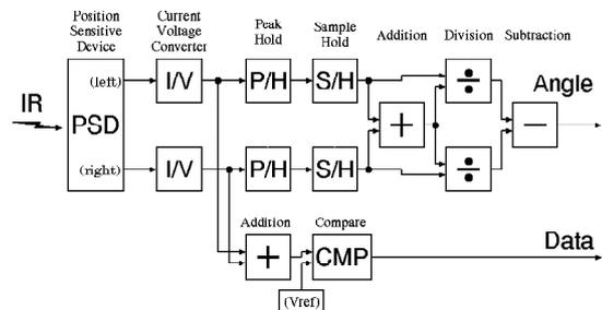
Fig. 12. Block diagram of analog computing circuit.
