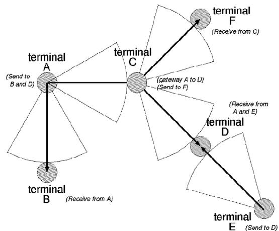
Fig. 8. The mobile robot communication network.
