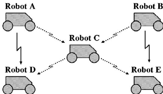
Fig. 1. Distributed communication structure.
