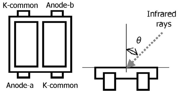
Fig. 11. Schematic view of the HAMAMATSU S6560 detector.
