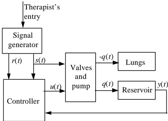
Fig. 2. Diagram of the functional blocks of the ventilator.
