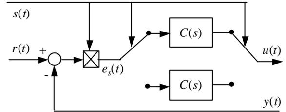
Fig. 4. The proposed scheme for a ventilation cycle of 2 sequences. The switches are driven by  $s(t)$ .
