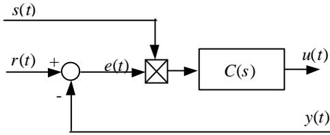
Fig. 4. The control scheme with a classical controller.
