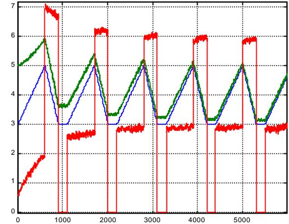
Fig. 5. Typical simulation results of liquid level (V) signal, reference signal (V) and command signal (V) versus the time in seconds.
