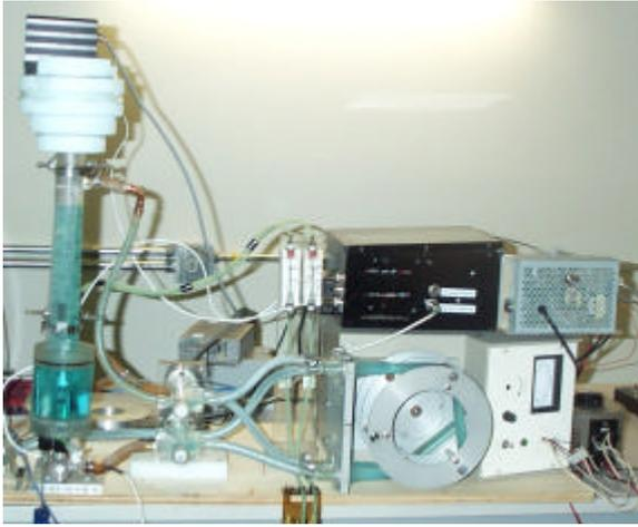
Fig. 1. The prototype of total liquid ventilator.
