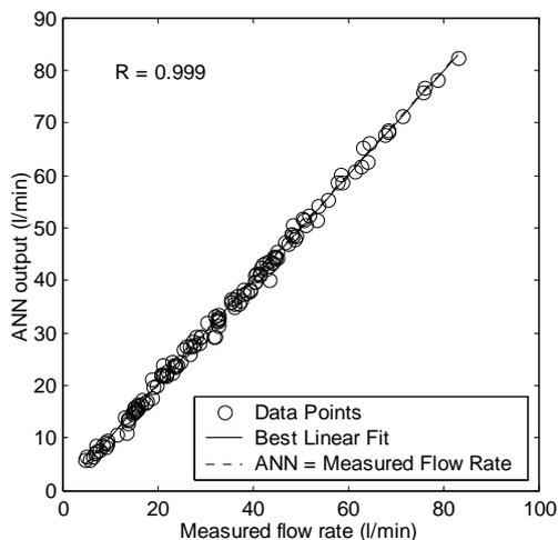
Fig. 8. Correlation between measured flow rate and provided by the ANN 2.
