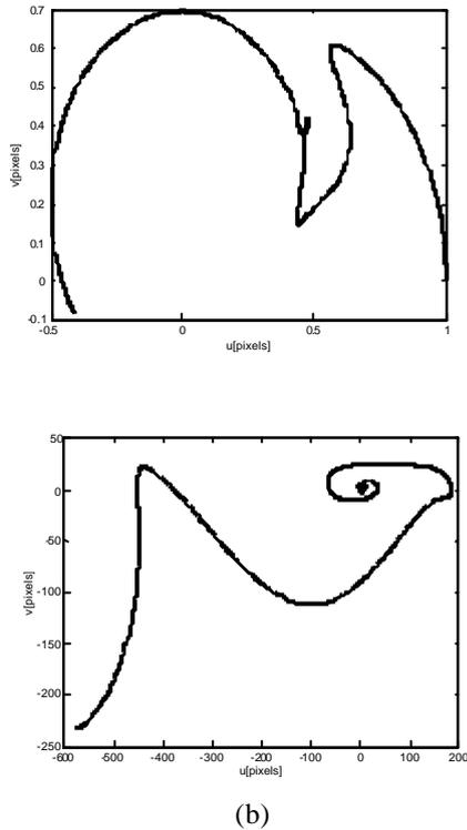
Fig.8. Experiment 2: Tracking. Simulation(a). Path of the camera in the robot workplane (b) Feature position trajectory in image plane
