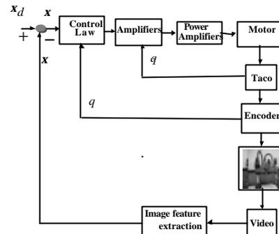
Fig. 4 Block diagram of image based visual servoing system.
