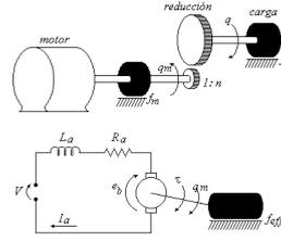
Fig. 3. Electrical and mechanical motor model.
