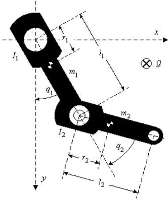
Fig. 1. 2 dof Scara Robot (BOSCH SR-800)
