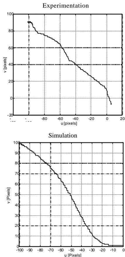
Fig. 6. Experiment 1: Comparison with Simulation. Feature position trajectory in image plane
