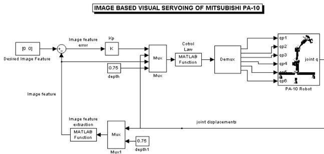
Fig. 9. Block diagram of image-based visual servoing system (Mitsubishi PA-10).
