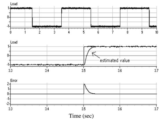
Fig. 9. Observed load and tracking error. Note when the load change its value, the observer response is fast.
