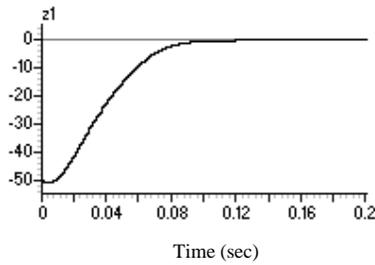
Fig. 5. Tracking error. Note that the error tends asymptotically to zero.
