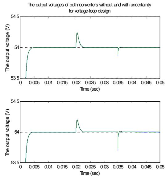
Fig. 10. The steady state and transient behavior of the output voltage of the voltage-loop in the presence of line & load disturbances without and with uncertainty, respectively.
