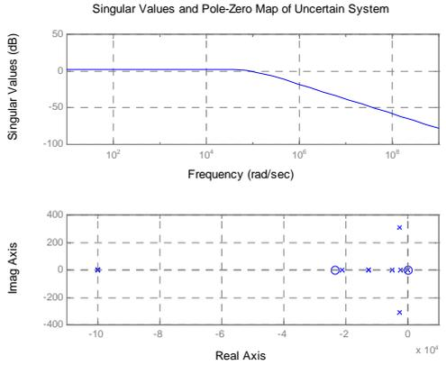
Fig. 9. The robust performance and stability tests for uncertain system, i.e.  $\bar{\sigma}(F) < \gamma$  for all  $\omega$  and  $F$  has all poles in LHP.
