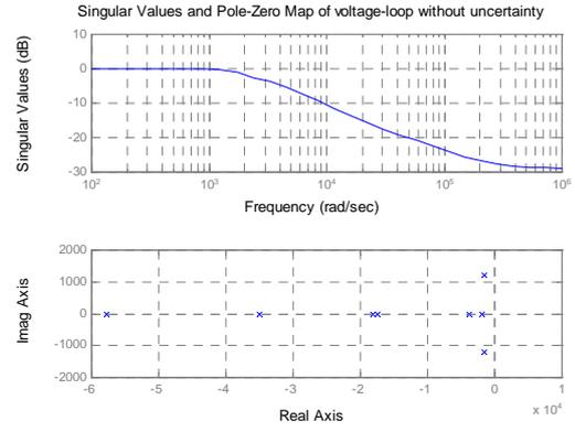
Fig. 6. The nominal performance and stability tests for voltage-loop, i.e.  $\bar{\sigma}(N_{v11}) < 1$  for all  $\omega$  and  $N_v$  has all poles in LHP.
