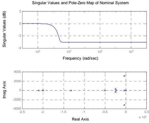
Fig. 8. The nominal performance and stability tests for the overall system, i.e.  $\bar{\sigma}(N_{11}) < \gamma$  for all  $\omega$  and  $N$  has all poles in LHP.
