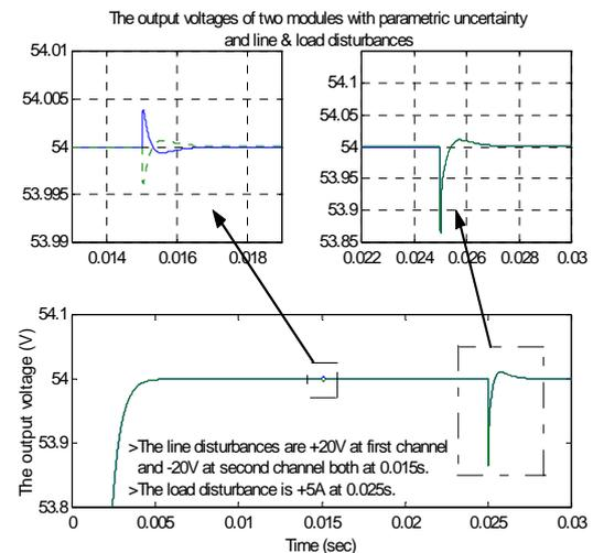
Fig. 11. The steady state and transient behavior of the output voltages in the presence of line & load disturbances with uncertainty.
