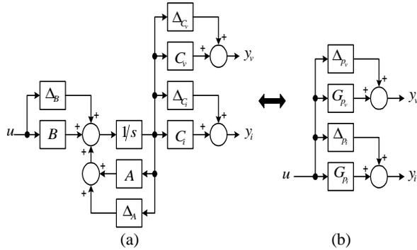
Fig. 3. The parametric uncertainty in state-space representation and its equivalent that inserts into the control system of Fig. 2.
