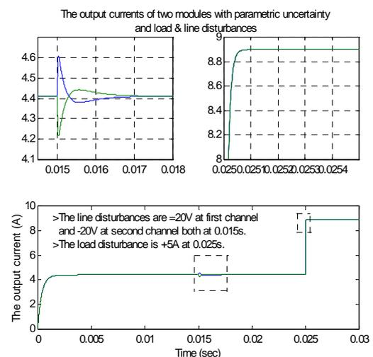
Fig. 12. The steady state and transient behavior of the output currents in the presence of line & load disturbances with uncertainty.
