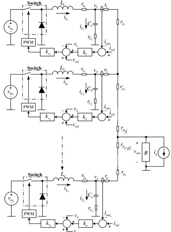
Fig. 1. Paralleled DC/DC converters feeding a resistive load with cascaded controllers for voltage- and current-loops.
