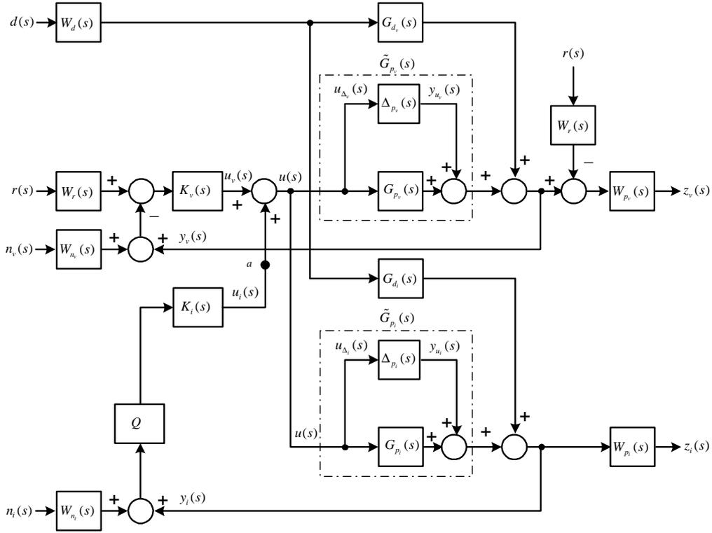
Fig. 2. The control configuration of paralleled DC/DC converters including all uncertainties. The control of voltage-loop is considered when it is isolated from the current-loop by breaking the connection at point *a*.
