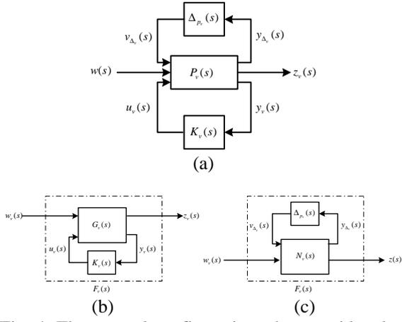
Fig. 4. The general configurations that considered to design and analysis the voltage-loop control of paralleled DC/DC converters in the presence of uncertainty.
