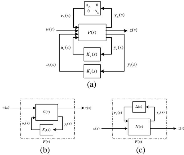
Fig. 5. The general configurations that considered to design and analysis the current-loop control of paralleled DC/DC converters in the presence of uncertainty.
