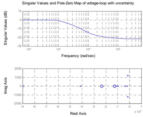
Fig. 7. The robust performance and stability tests for uncertain voltage-loop, i.e.  $\bar{\sigma}(F_v) < 1$  for all  $\omega$  and  $F_v$  has all poles in LHP
