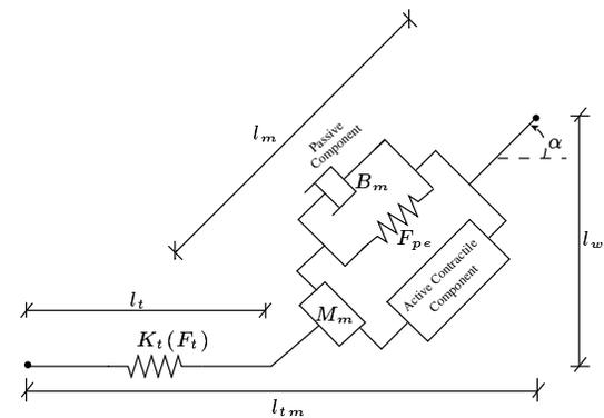
Fig. 2. Hill-type model of the musculotendon complex.
