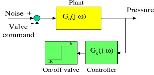
Fig. 2. Model of the controlled combustion process with on-off valves.
