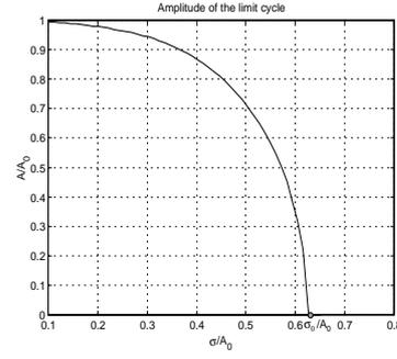
Fig. 3. The amplitude of the limit cycle in the presence of the Gaussian noise
