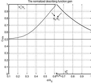
Fig. 4. Describing function gains in the presence of Gaussian noise
