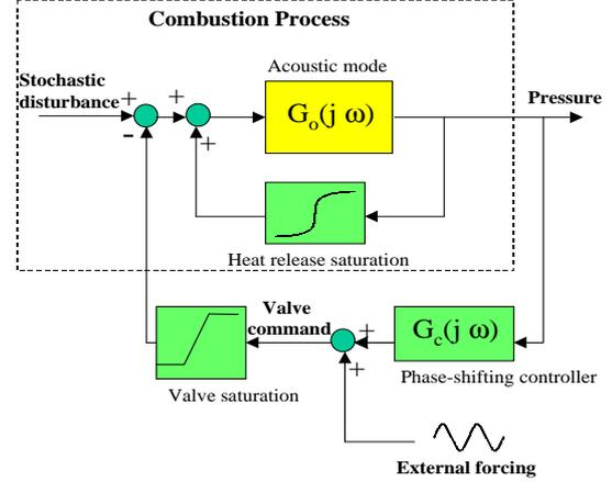
Fig. 1. Nonlinear model's block diagram
