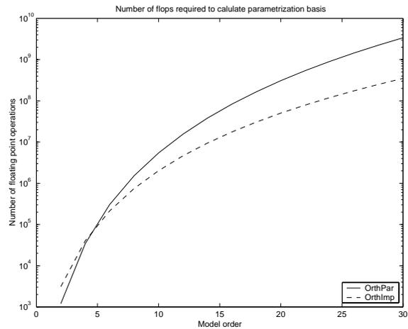
Fig. 1. The graph illustrates the number of floating points operations required for calculating the parametrization basis  $P$  for the OrthPar and the new OrthImp parametrizations.
