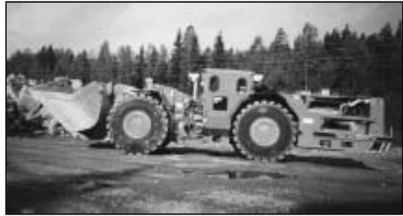
Fig 1. LHD machine Toro450D manufactured by Sandvik Tamrock Corporate.
