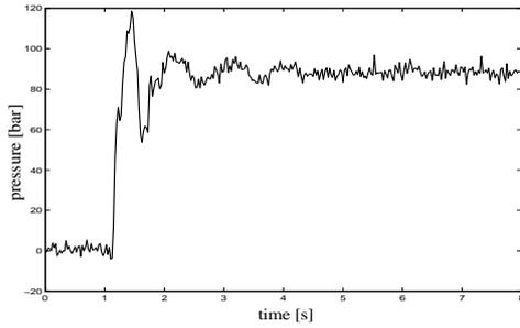
Fig 3. Upper pressure during boom lifting. Pressure at the other side of the cylinder piston makes a step down at the same time as the pressure value rises on the other side.
