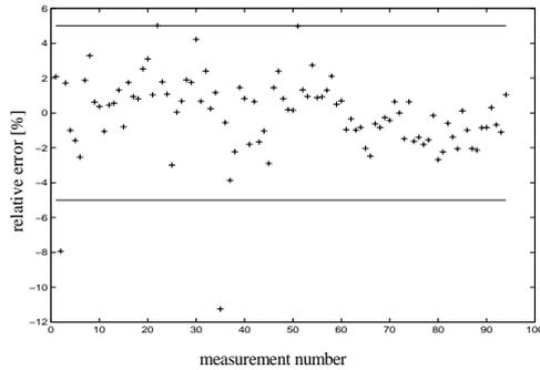
Fig 15. Relative error for the weighing results from the neural network.
