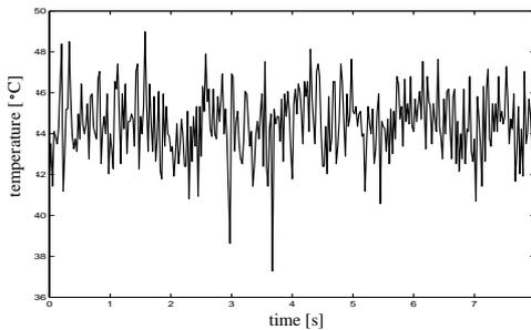
Fig 5. Temperature of hydraulic oil during weighing.
