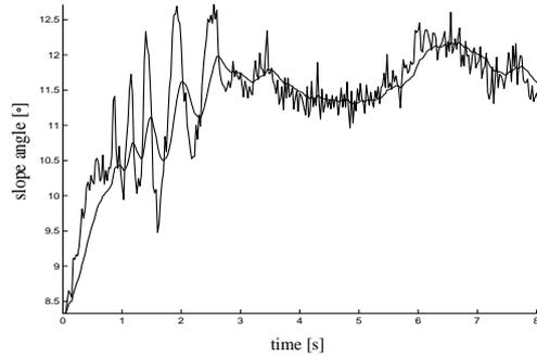
Fig 11. Kalman filter in estimating the slope angle.
