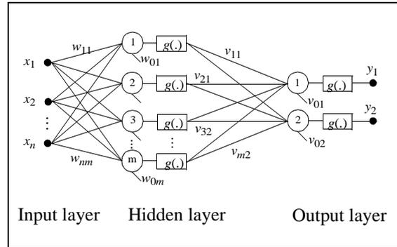
Fig 12. Example of MLP type of neural network.
