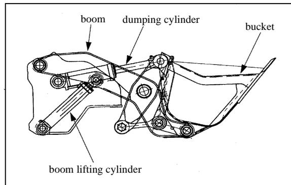
Fig 2. Structure of the machine front.
