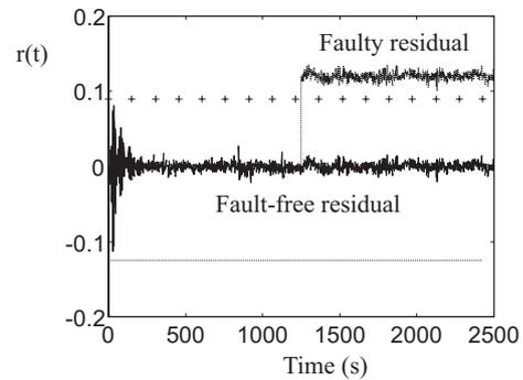
Fig. 3. Residuals for the signal  $\alpha(t)$  with de-coupling approach
