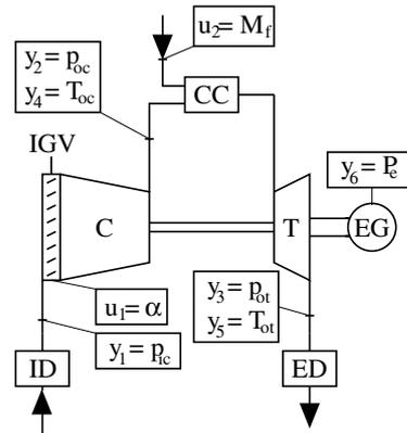
Fig. 1. Layout of the turbine model.
