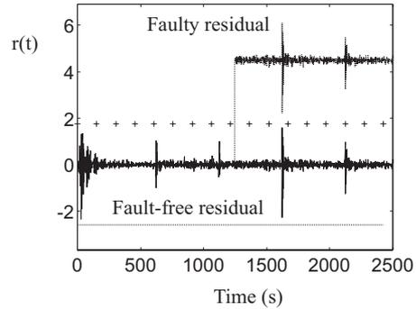
Fig. 2. Residuals for the actuator signal  $\alpha(t)$  without de-coupling procedure
