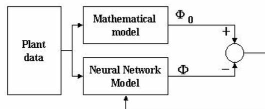
Fig. 4. Schematic diagram of learning method
