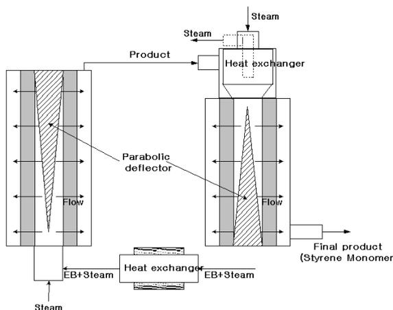
Fig. 1. Reactor configuration of current adiabatic radial flow reactor
