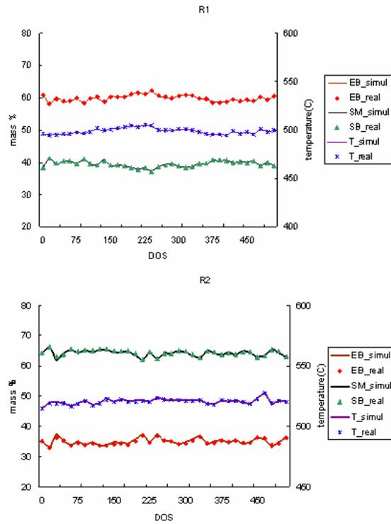
Fig 8. Comparison of simulation data and real plant data of reactors: a) reactor1, b) reactor2
