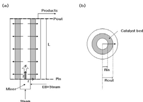
Fig. 2. Simplified reactor model and cross-sectional configuration
