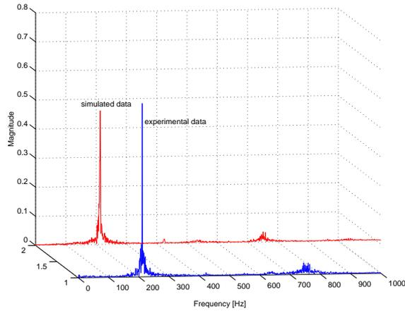
Fig. 6. Comparison of  $|FFT|$  of experimental data,  $p_t$ , and closed loop simulated data,  $\hat{p}_t$ , using a closed loop simulation measure.
