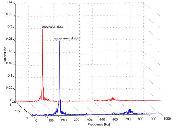
Fig. 5. Comparison of  $|FFT|$  of experimental data,  $p_t$ , and open loop predicted data,  $\hat{p}_t$ , using an open loop prediction error measure.
