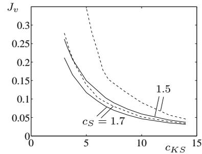
Fig. 5.  $J_v$  versus  $c_{KS}$  as obtained from Algorithm 1. The upper two curves are for  $c_S = 1.5$  and the lower two for  $c_S = 1.7$ . Solid: PID control. Dashed: PID weighted  $\mathcal{H}_\infty$  control.
