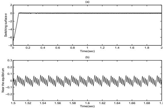
Fig. 5. System performance under conventional signum controller without unmodeled dynamics: (a) Switching surface; (b) Near the equilibrium.
