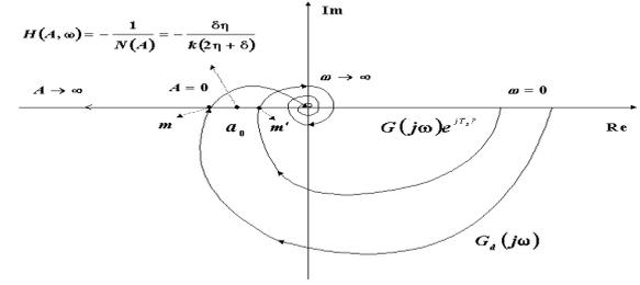
Fig. 4. Detection of a limit cycle in the case of a second order unmodeled dynamics and sampling delay.
