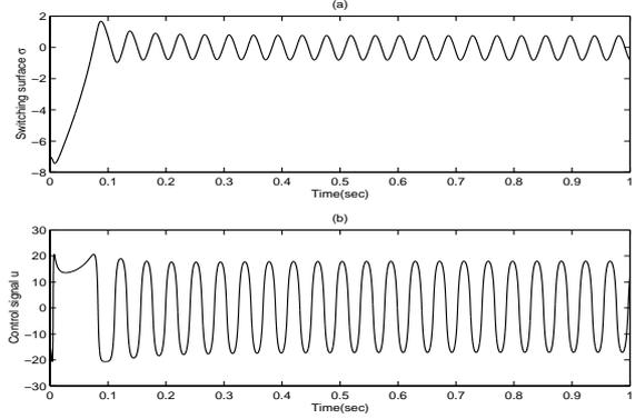
Fig. 7. System performance under the proposed fractional interpolation control scheme ( $\eta = 0.08$  and  $\delta = 1$ ) with the second order stable unmodeled dynamics  $D_1(s)D_2(s)$ : (a) Switching surface; (b) Control profile.
