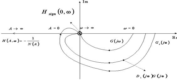
Fig. 2. Detections of the limit cycle in the DC servo motor.
