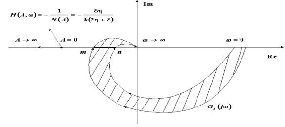
Fig. 3. Detection of a limit cycle in the case of a second order unmodeled dynamics.
