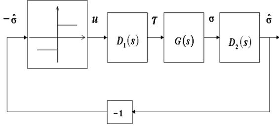
Fig. 1. Block diagram of the DC servo motor with signum function.
