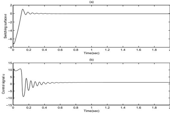
Fig. 9. System performance with proposed controller ( $\eta = 0.3$  and  $\delta = 1.5$ ) in the case of the second order stable unmodeled dynamics: (a) Switching surface; (b) Control profile.
