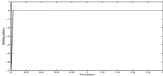
Fig. 6. The evolution of the switching surface under the proposed fractional interpolation scheme ( $\eta = 0.08$  and  $\delta = 1$ ).
