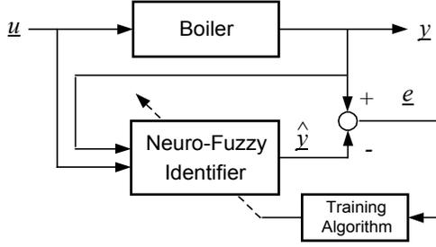
Fig. 2. Series-parallel identification.
