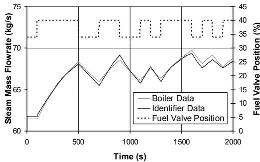
Fig.5. Steam mass flowrate of identifier and boiler in response to fuel valve deviation in low power.
