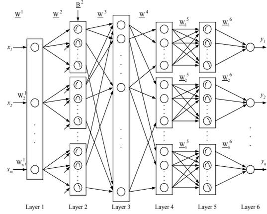
Fig. 2. Structure of neuro-fuzzy identifier
