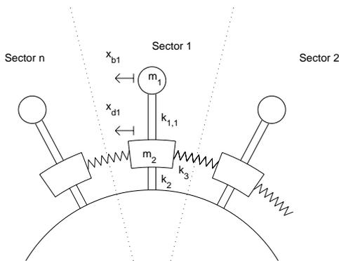
Fig. 2. Schematics of example rotor.
