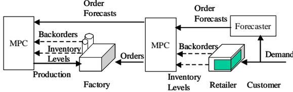
Fig. 3. Two-node network MPC information flows.
