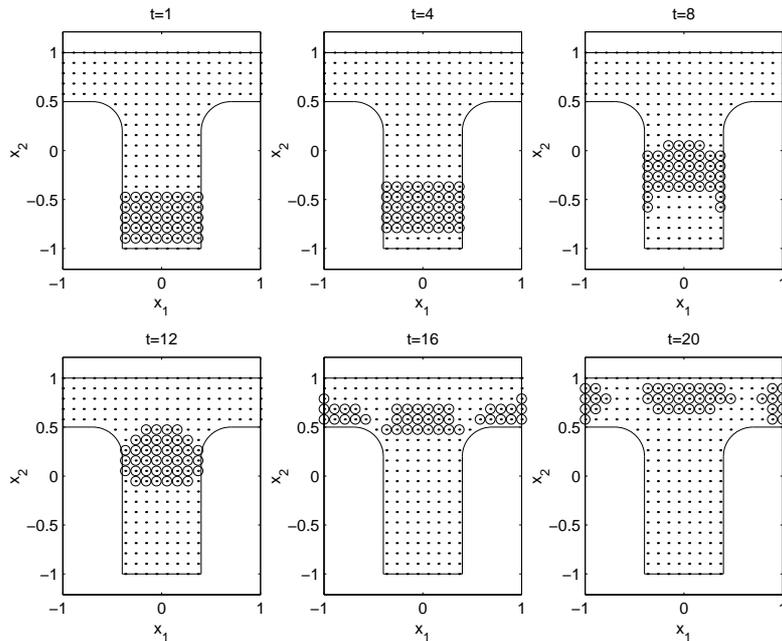
Fig. 2. Consecutive sensor configurations for the D-optimality criterion.
