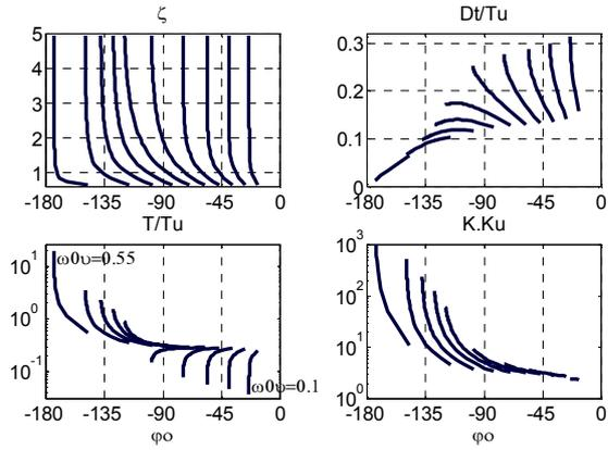
Fig. 3. ‘True’ SOPDT model parameters as a function of  $\varphi_0$  for different values of  $\omega_{0u}$ .
