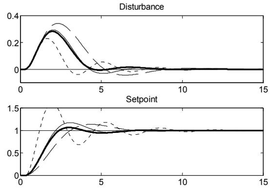
Fig. 6. Responses to setpoint and load disturbance changes for example 1 with PI control. Proposed (thick). PP method (---). Åström (---). Z-N (...).
