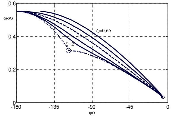
Fig. 2. Relationships between normalized parameters  $\varphi_0$  and  $\omega_{0u}$  for different values of  $\zeta$ , for the normalized SOPDT model (7).  $P_1$  (---).  $P_6$  (...).  $P_{a3}$  (-.-).  $P_5$  (O).  $P_{a4}$  (o).
