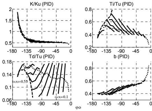
Fig. 5. PID control parameters as a function of  $\varphi_0$  for different values of  $\omega_{0u}$ . Integrating plants (---). Non-integrating plants (...).
