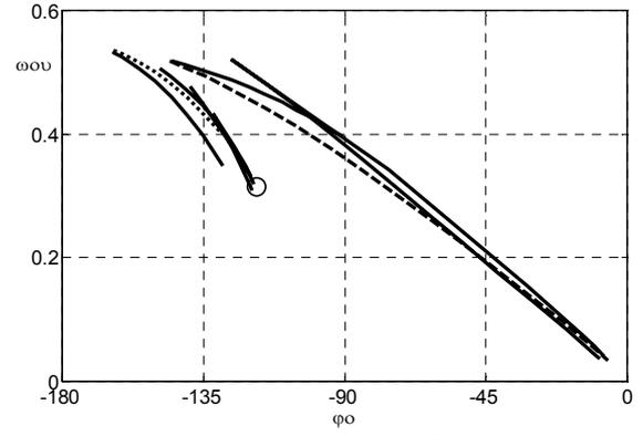
Fig. 1. Relationships between normalized parameters  $\varphi_0$  and  $\omega_{0u}$  for the test batch of process models.  $P_1$  (---); near it, non-integrating processes  $P_2$  to  $P_4$ ,  $P_6$  (...); near it, integrating processes  $P_7$  to  $P_{11}$  and  $P_5$  (O).
