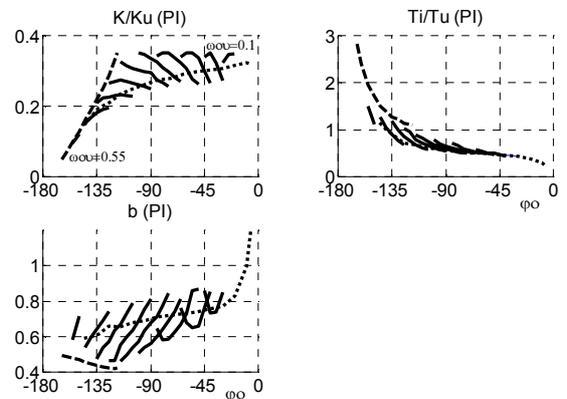
Fig. 4. PI control parameters as a function of  $\varphi_0$  for different values of  $\omega_{0u}$ . Integrating plants (---). Non-integrating plants (...).
