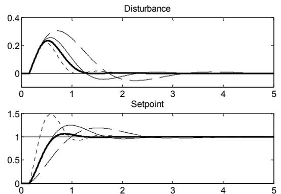
Fig. 7. Responses to setpoint and load disturbance changes for example 2 with PI control. Proposed (thick). PP method (---). Åström (---). Z-N (...).
