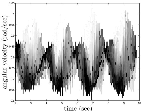
Fig. 2. Effect of torque pulsation on the motor angular velocity
