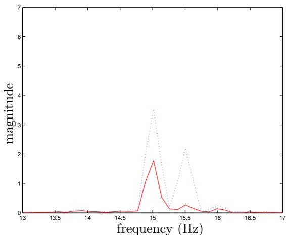
Fig. 7. Angular velocity spectrum for  $\omega = \pi/4$ , without compensation (dotted) and with compensation (solid)
