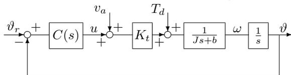
Fig. 1. DC Motor block diagram
