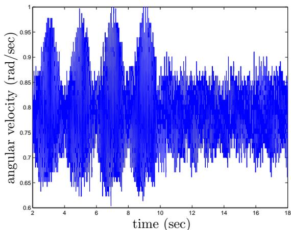
Fig. 6. Angular velocity for  $\omega = \pi/4$  with compensation applied at  $t = 10$  sec
