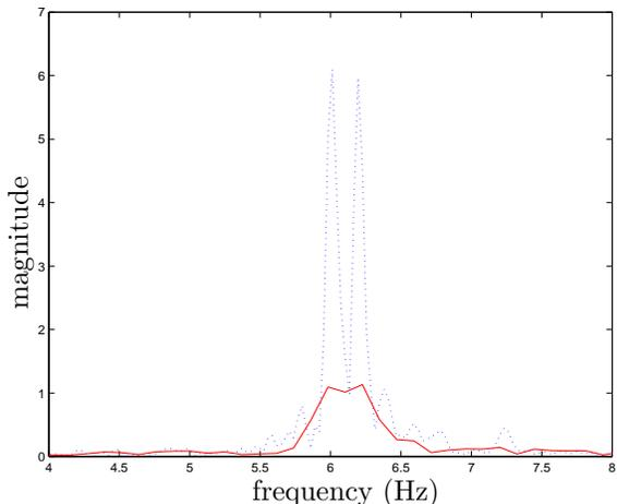
Fig. 5. Angular velocity spectrum for  $\omega = \pi/10$ , without compensation (dotted) and with compensation (solid)
