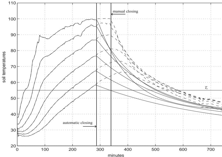
Fig. 6. Temperature behavior during treatment; - - - manually controlled and — automatic controlled. The control strategy allows to save 55 minutes of treatments, i.e. about 17% of the global costs.
