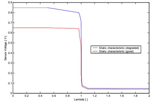
Figure 9: Oxygen sensor static characteristic: good and degraded.
