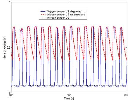
Figure 13: Oxygen sensors US fall time degraded, no degraded and DS sensor.
