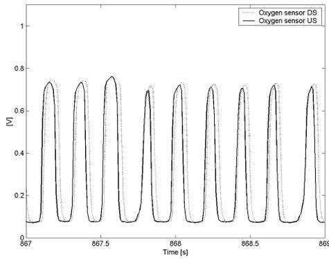
Figure 7: Oxygen sensors voltage outputs with a degraded TWC.
