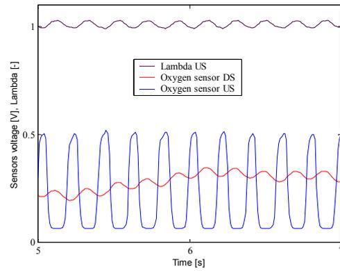
Figure 10: Oxygen sensors voltage outputs with a degraded US sensor, and actual  $\lambda$ .
