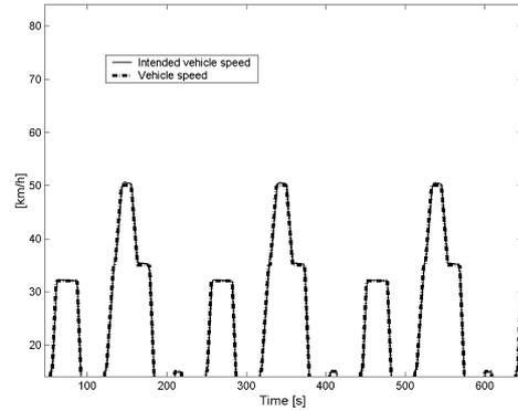
Figure 3: Velocity profile of NEDC, with TWC validation points.
