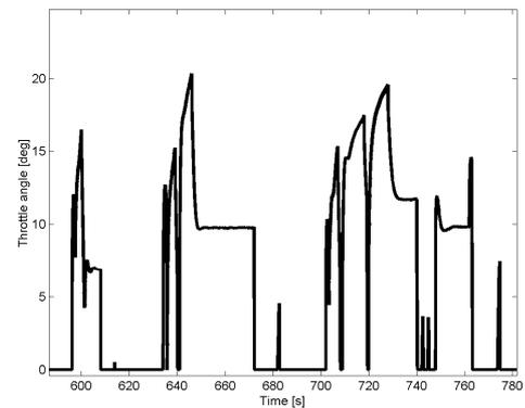
Figure 4: Throttle angle in urban part of NEDC.
