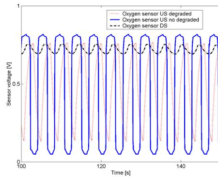
Figure 11: Oxygen sensors US frequency degraded, no degraded and DS sensor.
