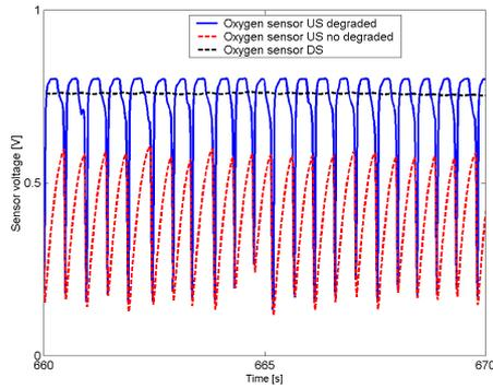
Figure 12: Oxygen sensors US rise time degraded, no degraded and DS sensor.
