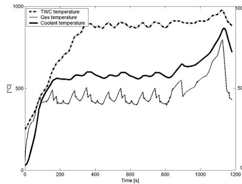
Figure 5: Temperature profiles of TWC, gas and coolant during NEDC.
