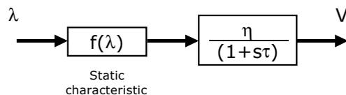
Figure 2: Lambda sensor block diagram mode
