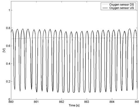
Figure 6: Oxygen sensors voltage outputs with a good TWC.
