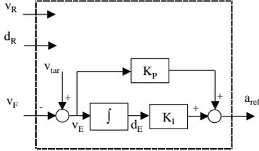
Fig. 3. GO and CRUISE phases reference generator.
