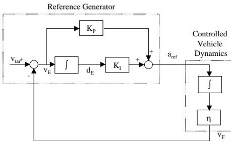
Fig. 4. Approximated controlled longitudinal vehicle dynamics and reference generation scheme.
