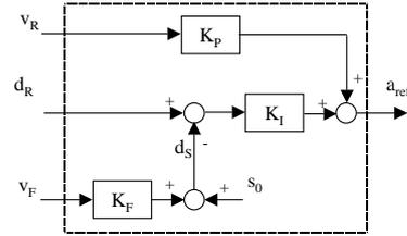
Fig. 5. TRACK phase reference generator.
