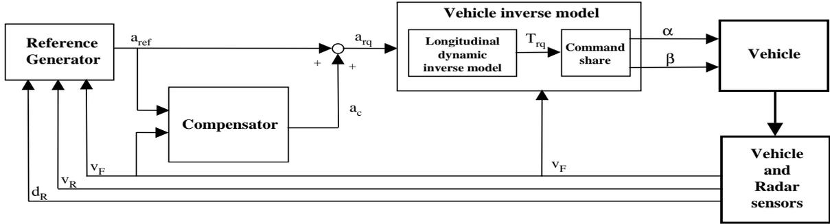
Fig. 1. Control structure.
