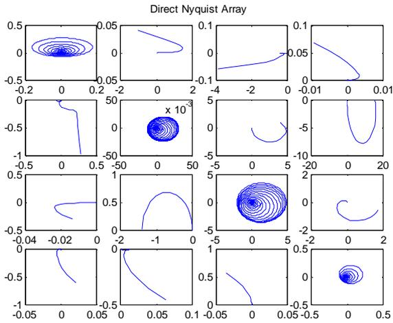
Figure 3: Direct Nyquist Array of the 4 x 4 gasifier
