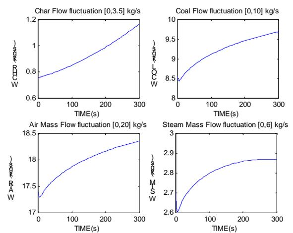
Figure 6: Gasifier outputs and inputs for a step pressure disturbance (100% load condition)
