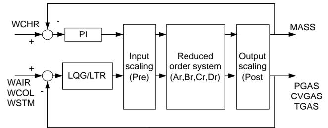
Figure 5: Final control structure
