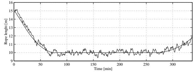
Fig. 4. Rope length with conventional model predictive control (solid) and with generalized mean. (dashed-dotted).
