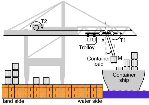
Fig. 2. Schematic picture of the container gantry crane
