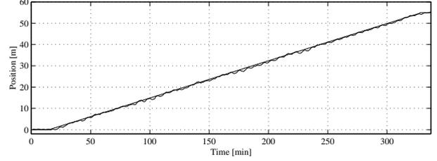
Fig. 3. Position with conventional model predictive control (solid) and with generalized mean (dashed-dotted).
