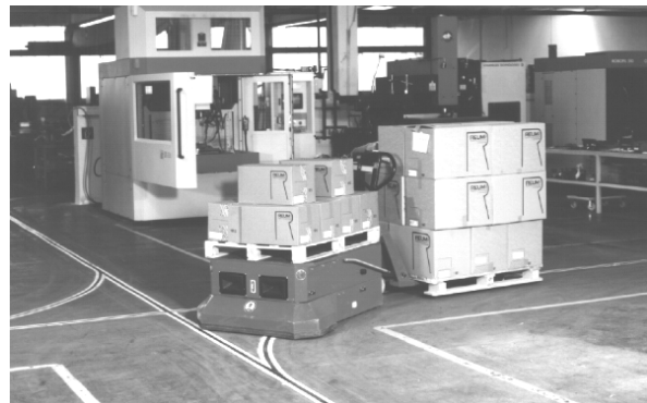
Fig. 1: An AGV coupled with a trailer, performing transport tasks in manu-facturing.
