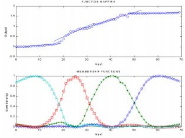
Fig. 2. AFCRC detection of real data structure (circle: experimental data, line: identified local model).
