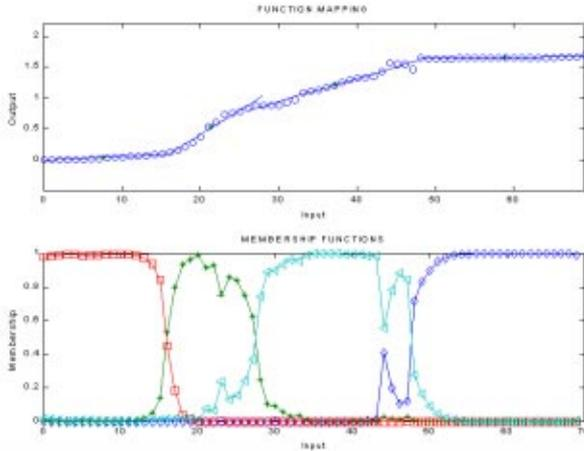
Fig. 1. GK detection of real data structure (circle: experimental data, line: identified local model).
