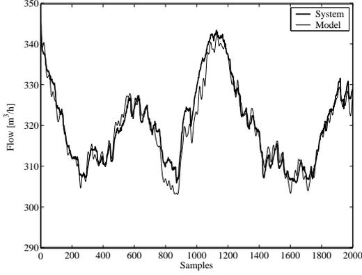
Fig. 5. Performance of Takagi-Sugeno N-F model for valve  $V_{51}$  (SSE /  $N.$  of samples = 6.774).
