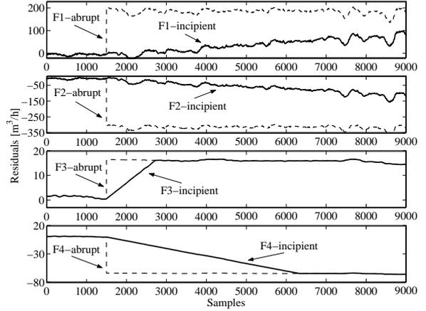
Fig. 6. Simulation of faults for both valves.
