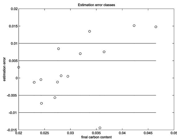
Fig. 5. Final carbon content estimate error vs final carbon content
