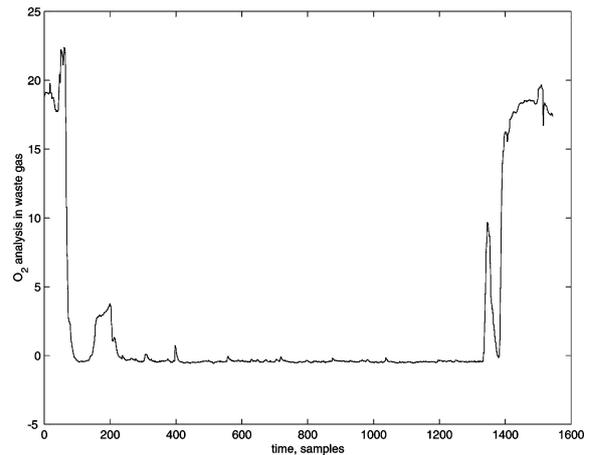
Fig. 10. Measured content of  $O_2$  in the waste gas for heat heat number 871. Notice the sharp peak just before the end of the process.
