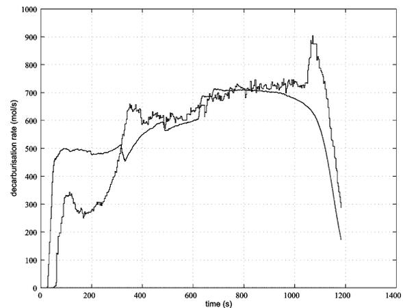
Fig. 7. Measured and estimated decarburization rate for heat number 902. Notice a drastic disturbance in the measured decarburization rate in the beginning of the downward slope.
