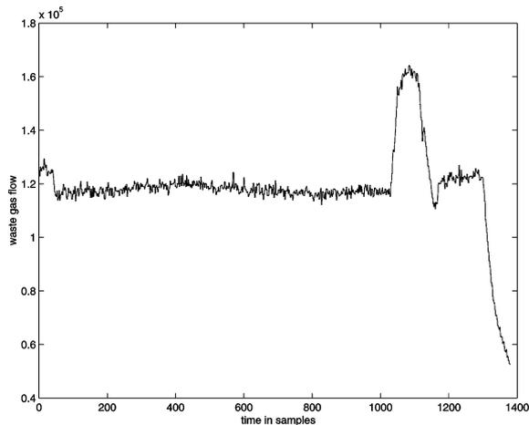
Fig. 8. Waste gas flow for heat number 902.
