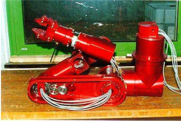
Fig. 6. The AMADEUS underwater arm requires over 150 wires to be integrated with the control architecture
