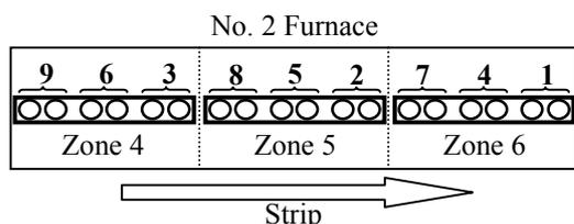
Fig. 4. Schematic of No. 2 Furnace illustrating arrangement of burners.
