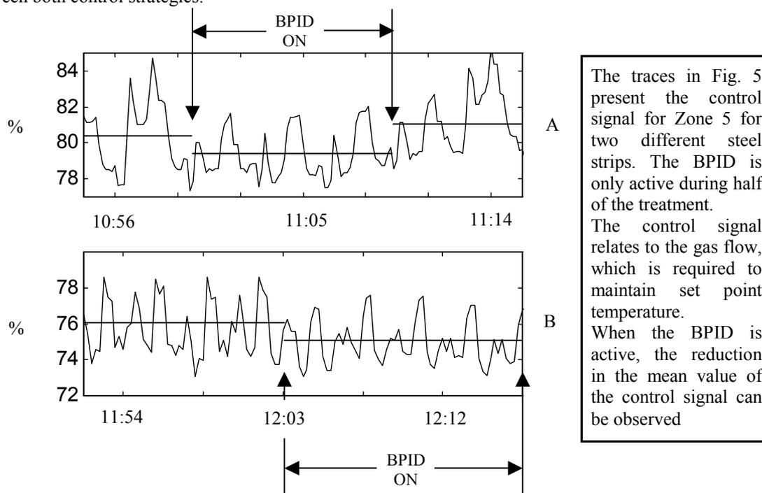
**Fig. 5. Control signal in % indicating periods of BPID operation.**
