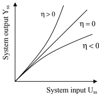
Fig. 1. Steady-state input/output characteristics of a bilinear system.
