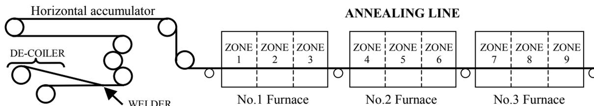
Fig. 3. Schematic of the Avesta Polarit annealing line.
