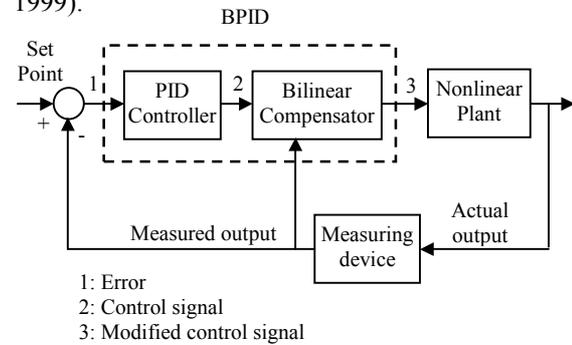
Fig. 2. Illustrating the configuration of the bilinear PID controller (BPID) implemented with the process.
