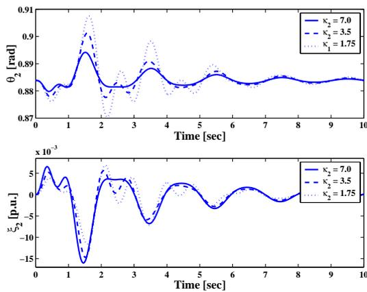
Fig. 7. Responses of phase angles and turbine outputs of the #2 machine
