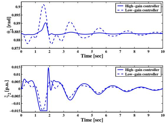
Fig. 9. Responses of phase angles and turbine outputs of the #2 machine
