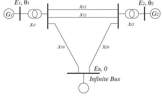
Fig. 1. Two-machine-infinite-bus system
