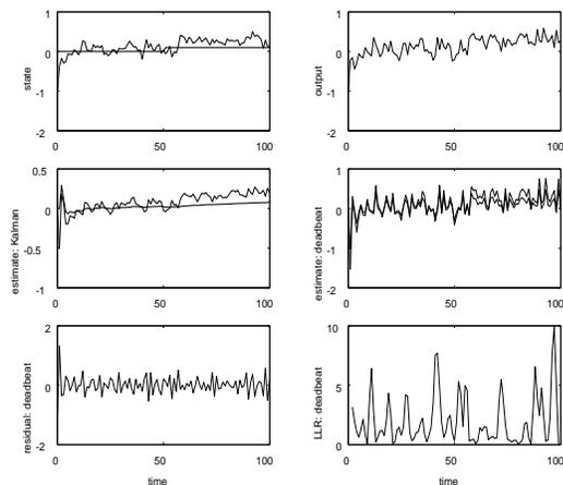
Fig. 1. GLR test for the jump  $\nu_1$  at time  $t_0 = 50$
