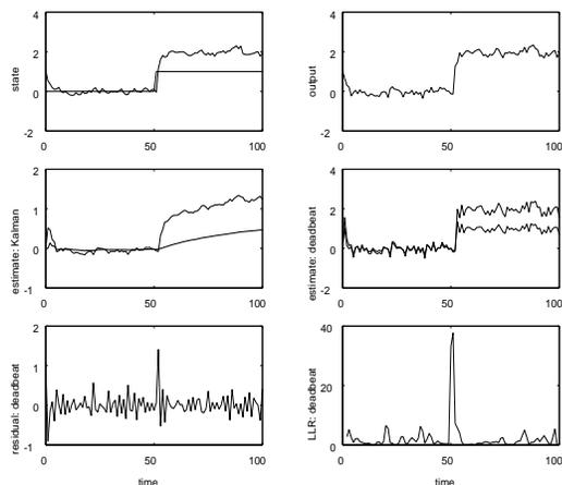
Fig. 2. GLR test for the jump  $\nu_2$  at time  $t_0 = 50$
