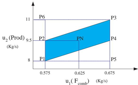
Fig. 4. Working area of control variables
