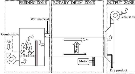
Fig. 1. Co-current rotary dryer
