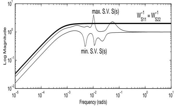
Fig. 9. Sensitivity singular value and  $W_S^{-1}$ . ( $\alpha_i = 0.5$ ,  $\beta_i = 10^{-4}$ ,  $\kappa_i = 0$ ,  $\omega_{T11} = 0.003$ )
