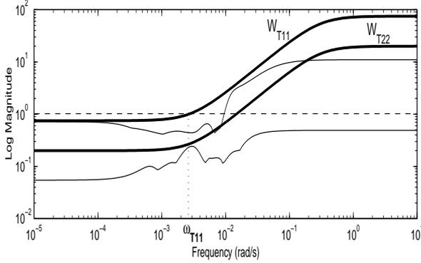
Fig. 8. Magnitude of the  $W_T$  weighting transfer functions.
