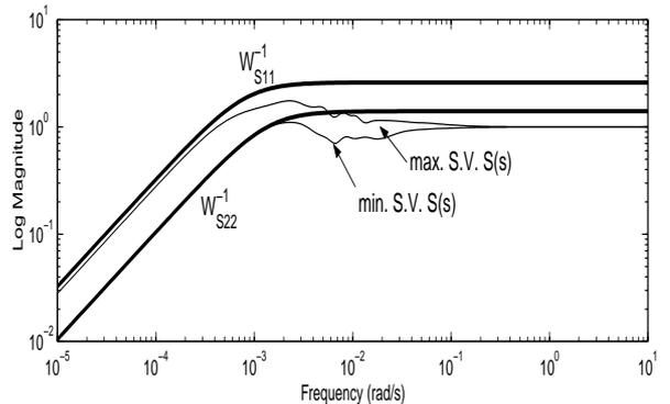
Fig. 11. Sensitivity singular value and  $W_S^{-1}$ . ( $\alpha_1 = 0.5$ ,  $\alpha_2 = 0.7$ ,  $\kappa_1 = 0$ ,  $\kappa_2 = 0.5$ )
