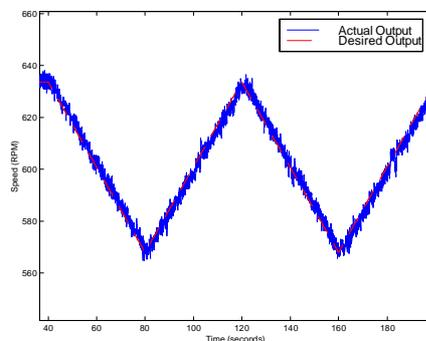
Fig. 3. System response to a ramp input (high-speed region).
