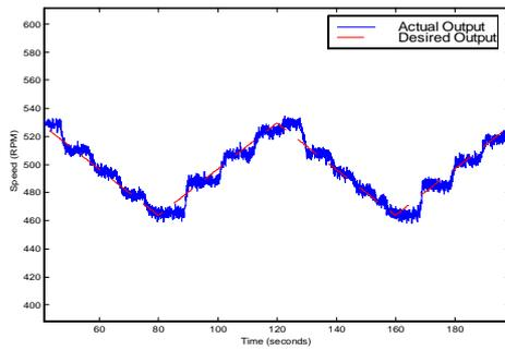
Fig. 5. System response to a ramp input (low-speed region).
