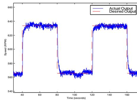
Fig. 2. System response to square wave input (high-speed region).
