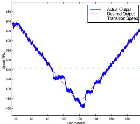
Fig. 7. System response to a ramp command operating in the high- and low-speed regions.
