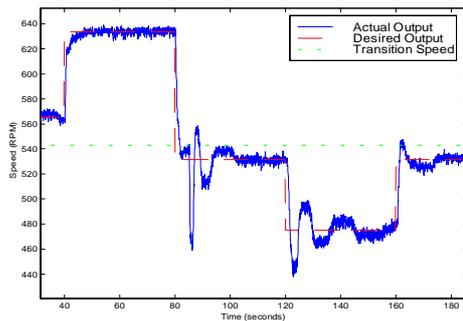
Fig. 6. System response to a square wave command operating in the high- and low-speed regions.
