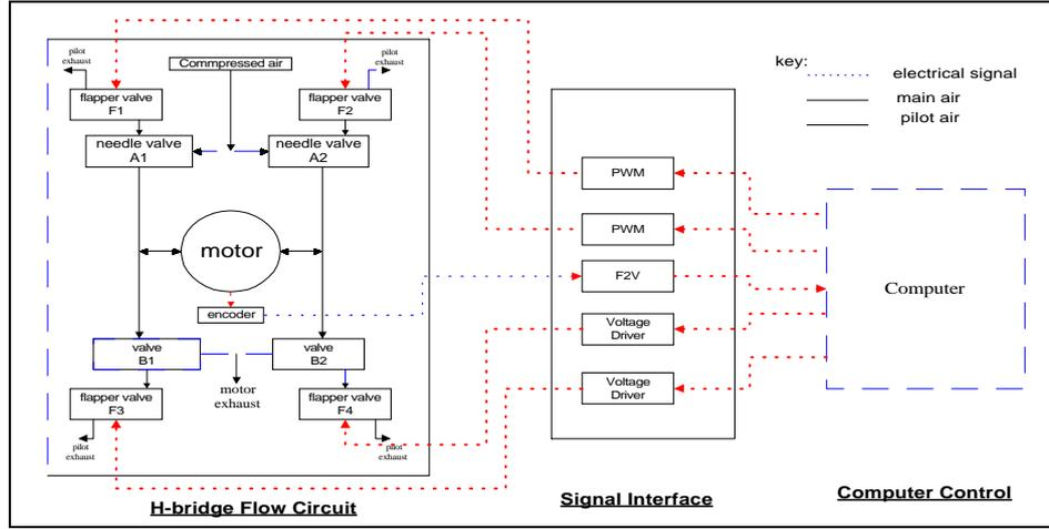
Fig. 1. Functional set-up of the H-bridge.
