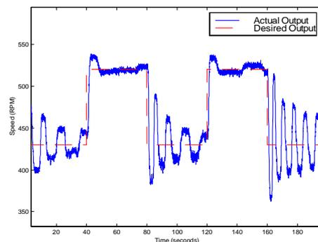
Fig. 4. System response to square wave input (low-speed region).
