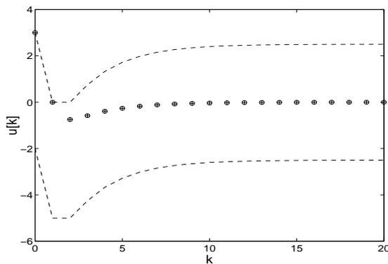
Fig. 4. Control sequence with  $\text{sat}_{U(x)}(-Kx)$  (circle) and with MPC (plus).
