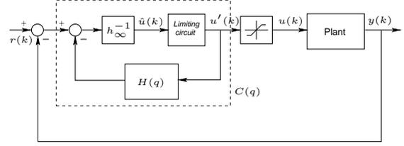
Fig. 1. General anti-windup scheme for input constraints.
