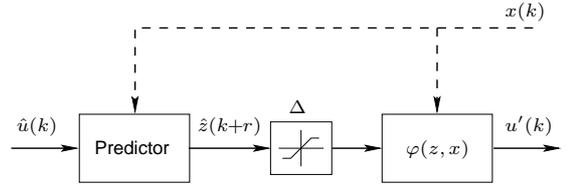
Fig. 2. Limiting circuit  $u'(k) = \text{sat}_{\mathbb{U}(x)}(\hat{u}(k))$  for the state constraint anti-windup scheme.
