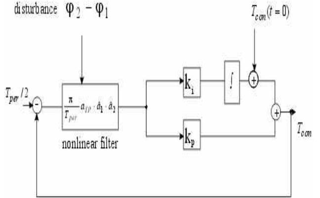
Fig. 1. Delay control system structure
