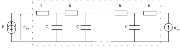
Figure 4 : Modeling of the heat transfer system
