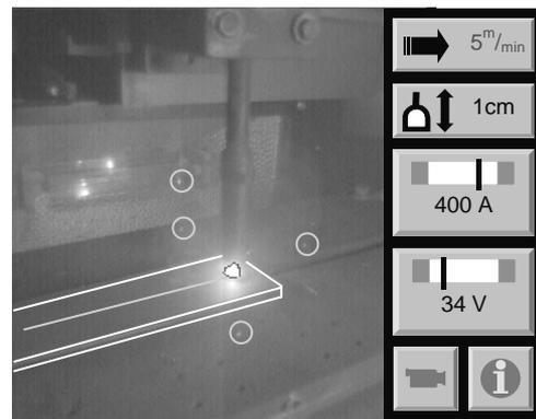
Fig. 8. Possible insertions: work piece geometry, welding seam, splashes, wire feed, height of the arc, welding current and welding voltage
