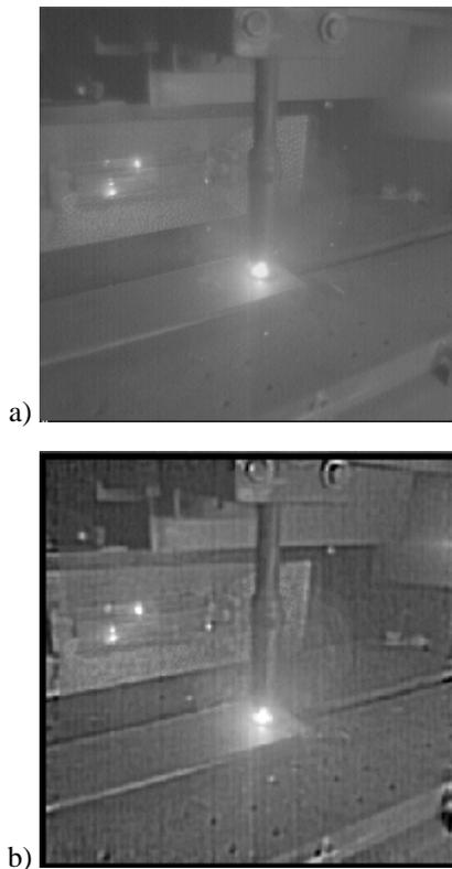
Fig. 6. (a) Original Image; (b) Result of adaptive contrast enhancement
