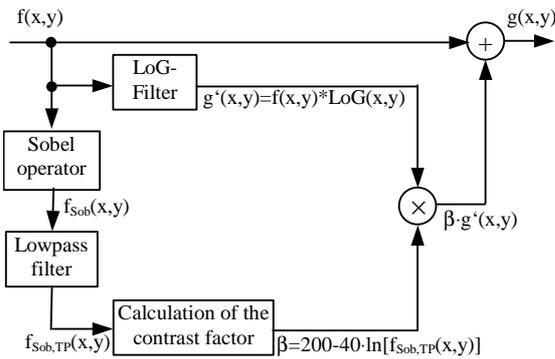
Fig. 5. Flow of the adaptive contrast enhancement procedure
