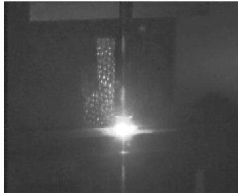
Fig. 1. Simulated view of the welder recorded with a CCD camera and standard protective glasses
