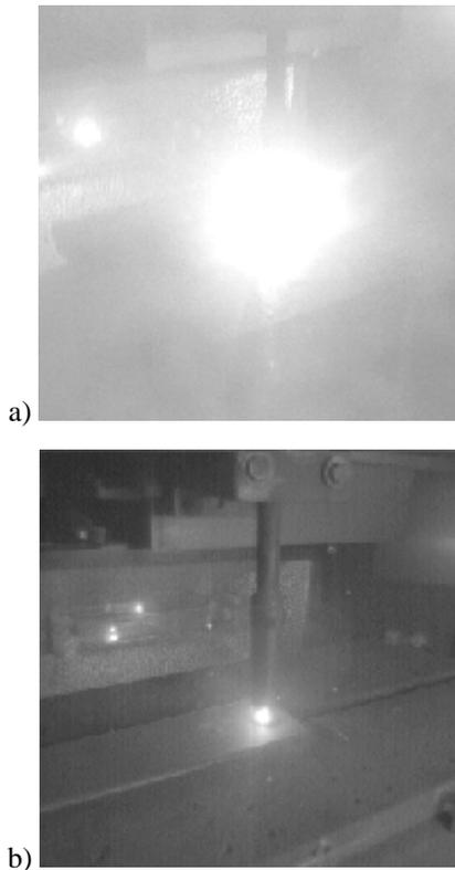
Fig. 4. Welding scene recorded with (a) CCD camera (b) HDRC camera
