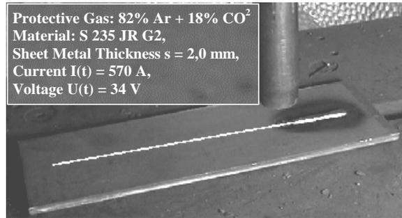
Fig. 7. Possible insertions: welding seam and welding parameters.
