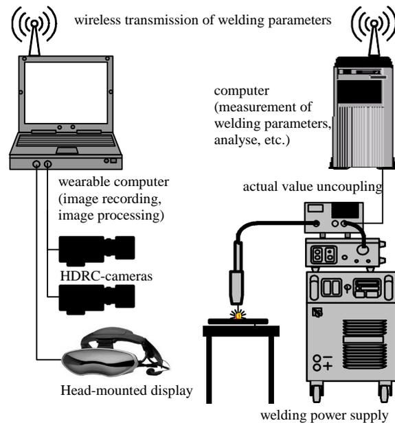
Fig. 2. Principle sketch of the system, depicted without the welding helmet
