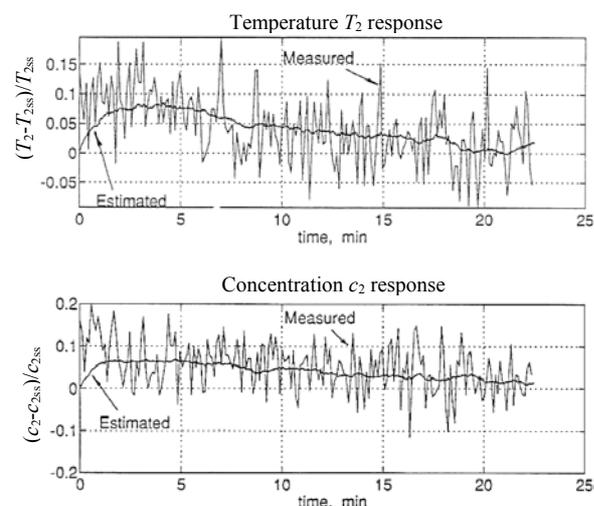
Fig. 4: Simulation of closed loop system response
