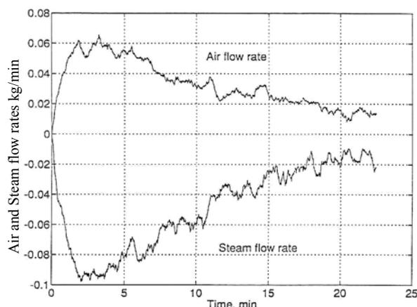
Fig. 5: Control efforts returning the process to steady state conditions from non-zero initial conditions
