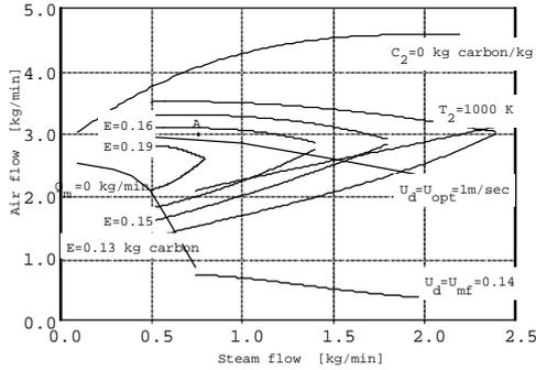
**Figure 3:** Efficiencies and constraints of the Judd gasifier model on the air-steam plane.
