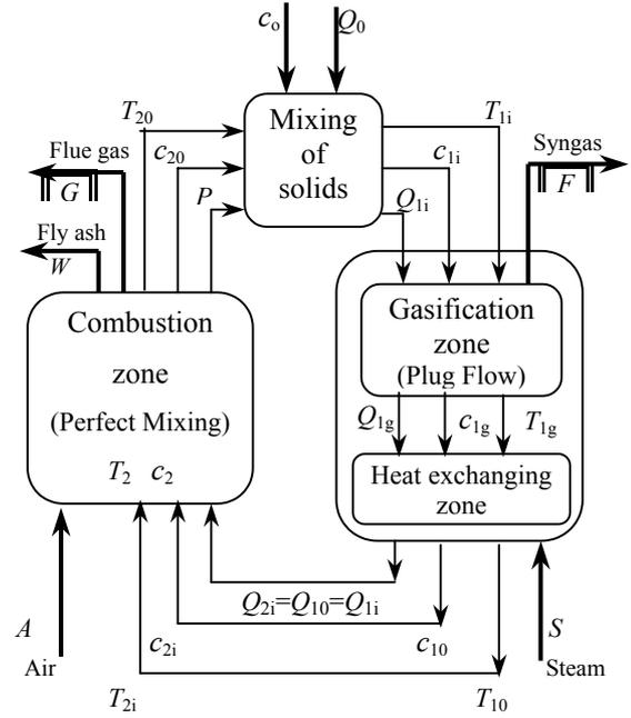
Figure 2: General scheme of the Judd gasifier model and nomenclature
