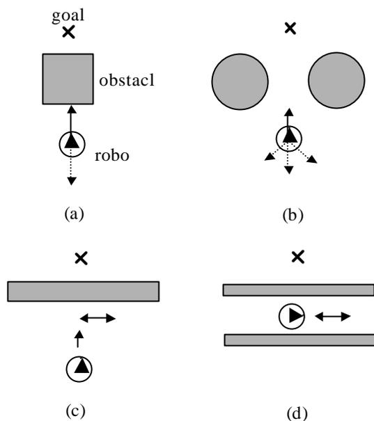
Fig. 6. Some traps in reactive navigation excluding box-canyon (a) deadlock by single obstacle (b) deadlock by multiple obstacles (c) cyclic moving in front of long obstacle (d) cyclic
