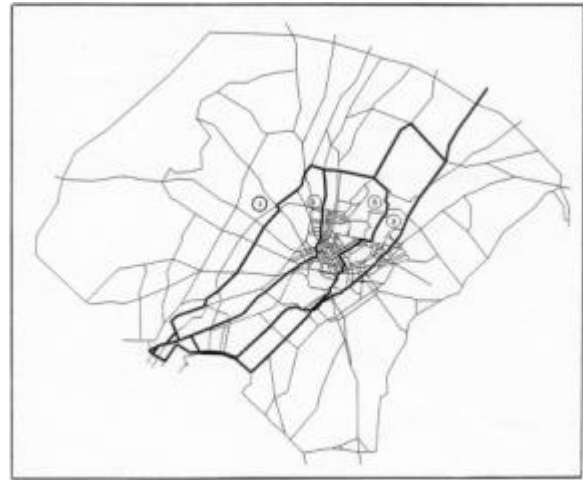
Fig. 3. Comparison of the first three minimum paths successively generated from the trip origin for updating period 5 minutes with the respective minimum path generated for updating period 15 minutes.
