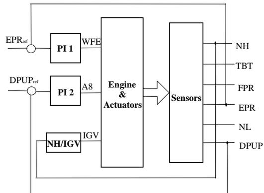
Fig. 3. Conceptual Spey model for the new configuration
