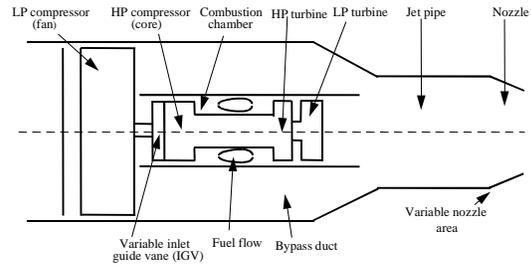
Fig. 1. The aero-engine
